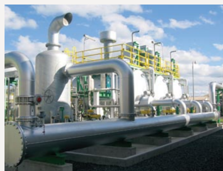
A facility for recovering volatile organic compounds prevents air pollution by various methods, such as concentration and adsorption.
