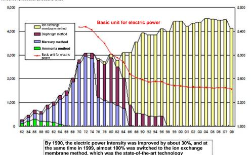
Fig. 11. Changes in energy intensity in the manufacturing processes of ethylene and caustic soda in Japan
