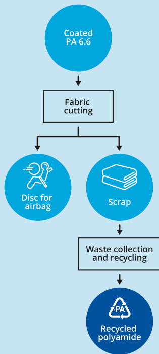
Figure 13: Recovery of high-quality polyamide from the scraps resulting from coated disks used to manufacture car airbags
